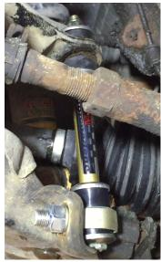
by simply tightening the vertical bolt until zero clearance between nut and Stainless Steel washer. Continue to tighten an additional 1.5-2.5 turns to set proper busing compression. If you continue to compress the sway bar links you will notice the lower axle mount bushings will begin to swell growing increasingly larger in diameter. Very little to no bushing compression is ideal. See detailed images bellow as a guide.
