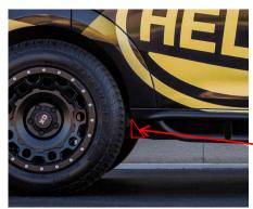
a) With 28.0" diameter or larger tires the tire will interfere with the front lower edge of the plastic rocker cover. Slight trimming may be necessary to eliminate this interference. See Figure #3
