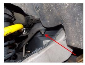
Figure 4: Sub-Frame Bolt (4 total)
