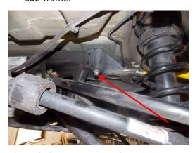
Figure 3: Sub-Frame Bolt (4 total)
