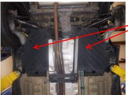
3. Remove the two (left hand and right hand) plastic underbelly panels located before the front axle.
