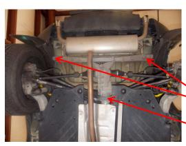
6. <u>4WD VEHICLES ONLY:</u> Remove the two bolts attaching the aluminum rear cross member to the main body structure. (16mm socket). This cross member is located at the very rear section of the vehicle behind the rear axle and is used on ALL4 Countryman only.
