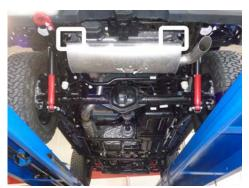
4. Loosen clamp then remove muffler from vehicle. Place it next to **tailpipe (3)** and transfer driver mount over.
