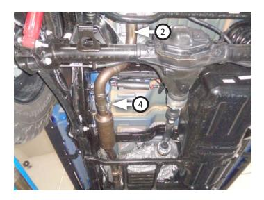
10. Place **clamp (4)** onto slip-fit of tailpipe then connect it to rear inlet pipe. Fasten mount to frame with bolts (x2) (removed step 3). Tighten clamp just enough to allow for adjustment.
