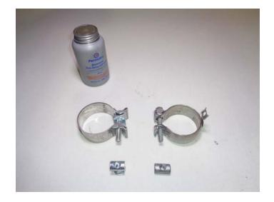
8. Place factory clamp (removed step 11) onto **muffler** (1), then connect it to factory pipe. Tighten clamp just enough to allow for adjustment.
