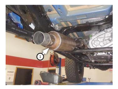
Place clamp (4) onto muffler outlet then connect rear inlet pipe (2) into it with bend oriented over axle.
