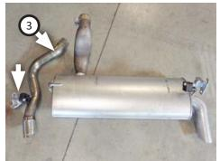
5. Remove factory rear of resonator assembly from rubber isolator then loosen bolt on clamp at inlet clamp.
