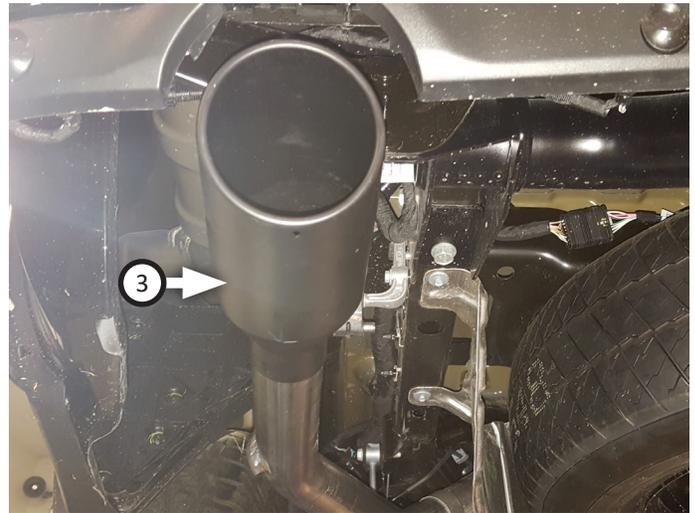
10. Adjust exhaust components for fit; maintaining ½" clearance and compensating for suspension, travel and vibration, then tighten all clamps. Finally, fit (x2) **hanger keepers (5)** onto each sideways hanger.
