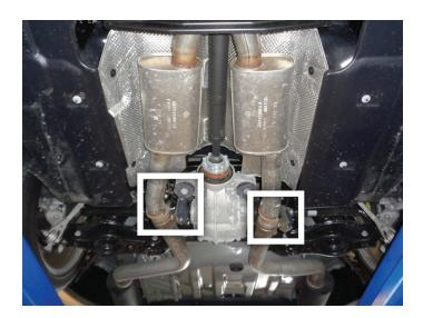
Unclip grounding strap and slide wire hanger out of rubber isolator on driver side tailpipe. Next, unbolt mount, flip it around and reinstall. Repeat step for passenger side tailpipe.
