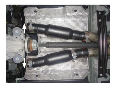
15. Place left and right tailpipes into muffler outlets while seating wire hangers in rubber isolators. Then reconnect exhaust valve actuators and clip in grounding wires.
