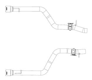
13. Place (x2) clamps (5) onto scavenger pipe (1) then connect it to front pipes. Tighten clamps enough to allow for adjustment. Re-install nuts (x8) and braces supports (removed step 6).
