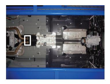
8. Remove nuts (x3) then detach actuator and spring from mount on driver side tailpipe. Retain actuator and spring for re-use. Repeat step for passenger side tailpipe.
