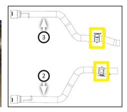
11. Place driver side actuator onto left tailpipe valve bracket with (x3) **flat washers (11)** in between. Then secure components with (x3) **screws (10)**. Repeat step on right tailpipe (removed step 8).
