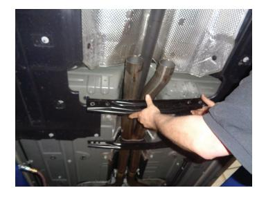
14. Place (x4) clamps (6) onto both mufflers (4) then connect them to scavenger outlets. Tighten clamps just enough to allow for adjustment.
