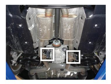
6. Remove nuts (x8) to uninstall braces supporting rear pipes. Retain nuts and braces for re-use.
