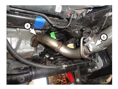
13. Place clamp (6) onto muffler (5) then connect it to rear inlet pipe. Support muffler, then ensure all connections are completely seated.
