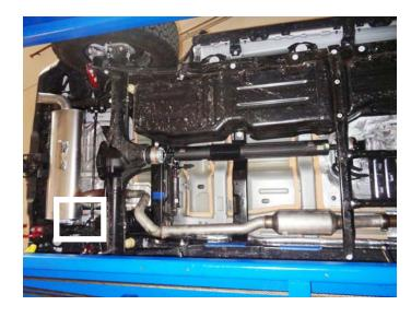
4. Remove bolts (x2) from mount on passenger side above muffler.
