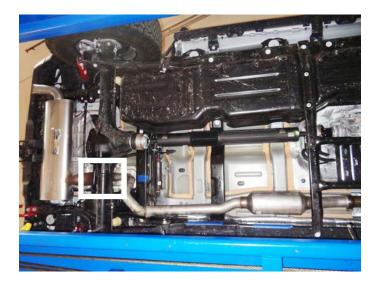
6. Remove muffler from vehicle. Place stock muffler next to Outlaw muffler oriented in the same direction, then transfer mounts (x2) over.
