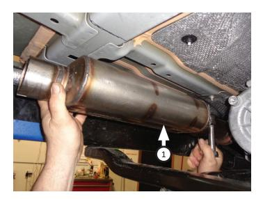
11. Place **clamp (5)** onto resonator then connect front pipe to it. Make sure front pipe bend is oriented upwards, then tighten clamp just enough to allow for adjustment.
