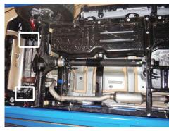
4. Loosen clamp at muffler inlet connection above rear axle then remove muffler from vehicle.
