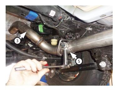
11. Place **clamp (5)** onto tailpipe, then connect it to over-axle pipe. Make sure tailpipe bend curves over suspension components, ensure connections are completely seated and tighten clamp.
