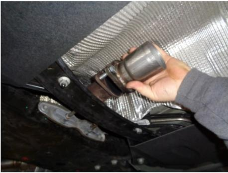
4) Using the 3/8" bolts, nuts and washers provided, bolt adapter assembly **873TBS** to the back of the flex pipe flange. Be sure to re-install the gasket. Tighten securely.
