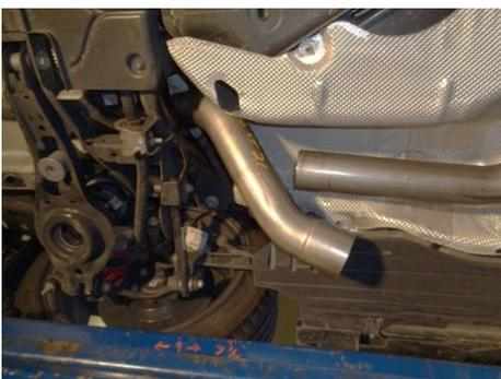
7) Place a supplied clamp onto the back of the intermediate pipe. Then place over-axle pipe **#26685S** into position from the front of the rear axle, and slip it onto the back of the intermediate pipe. Tighten the clamp enough to hold, but still allow for adjustment
