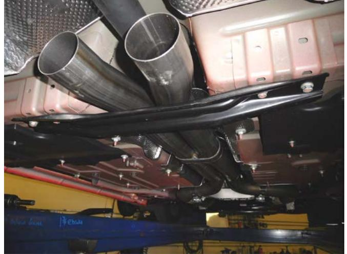
4) Place a supplied 3" clamp onto the inlet neck of both mufflers. Slide the mufflers onto the back of the Scavenger pipe assembly about 1-3/4" and support with stands. Level the mufflers and tighten the clamps enough to hold, but still allow for adjustment.
