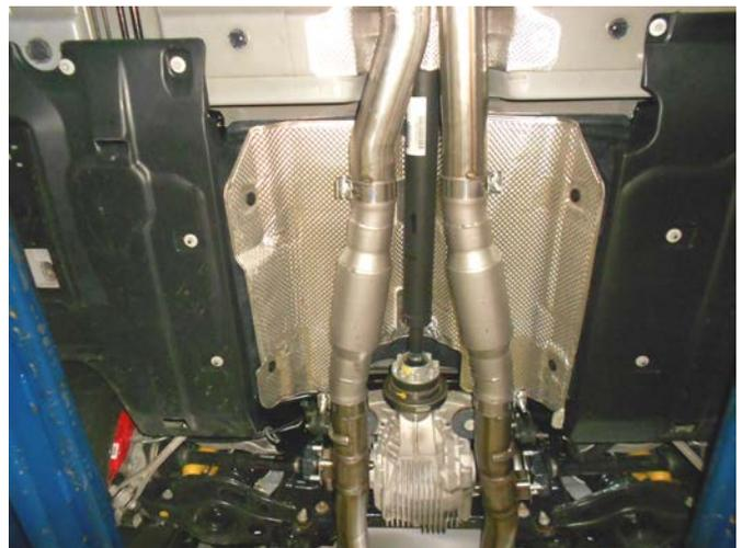
5) Place a supplied clamp onto the left muffler outlet. Place the left tailpipe **# 26654S** into position and starting from the rear, connect the hangers on the tailpipe to the rubber mounts on the vehicle. Slide the tailpipe fully into the muffler outlet and adjust the tailpipe so that the end of the pipe is centered in the factory exhaust bezel. See photo below. Tighten clamp enough to hold, but still allow for adjustment. Repeat this step for right tailpipe **# 26652S**.
