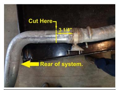
On the drivers' side of the system, Measure back 3 ¼" from the cast body of the exhaust valve and make a mark. Using a hacksaw or sawsall, cut the pipe through on this mark. After cutting, remove any burrs from the end of the pipe using a file or die grinder.
