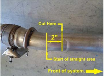
At the front of the drivers' side valve, locate the start of the straight area and measure forward 2". Make a mark. Using a hacksaw or sawsall, cut the pipe through on this mark. After cutting, remove any burrs from the end of the pipe using a file or die grinder.
