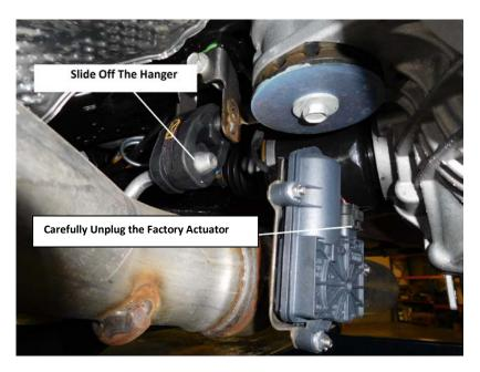
4) Slide the two hangers on each tailpipe out of the rubber mounts on the vehicle and unclip the grounding strap from the rear hanger on the right side of the vehicle. The stock system will come out as one large unit. Carefully lower the stands at the rear of the vehicle and with the help of an assistant slide the system back off of the head pipes and lower the system from the vehicle.
