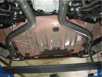
5) Reconnect the two electrical plugs removed in step 3 of the removal instructions back onto the tailpipe actuators.
