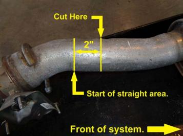
At the front of the passenger side valve, locate the start of the straight area and measure forward 2". Make a mark. Using a hacksaw or sawsall, cut the pipe through on this mark. After cutting, remove any burrs from the end of the pipe using a file or die grinder.
