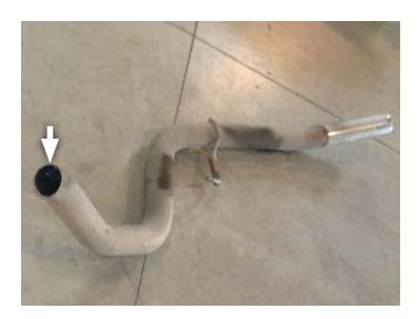
4. Disassemble wire hangers from isolators on vehicle, loosen clamp at muffler inlet connection then remove muffler and set aside.
