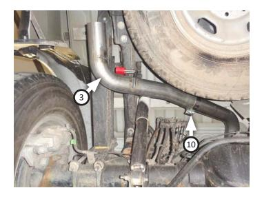
11. Place (x2) clamps (10) onto tailpipes then connect (x2) side exit pipes (6) to them.
