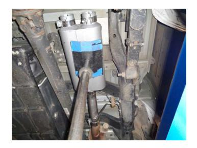
8. Remove bolts (x2) indicated below and use them to secure **left rear hanger (9)** onto vehicle frame. Then install **rubber hanger (11)** as shown.
