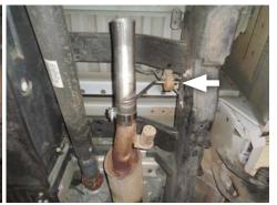
7. Place (x3) **clamps (10)** onto **muffler (2)** then connect it to inlet pipe. Tighten clamp just enough to allow for adjustment.
