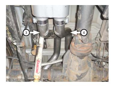
10. Place clamp (10) onto left rear tailpipe (5) and connect it to left front tailpipe. Insert wire hanger into isolator and tighten clamp just enough to allow for adjustment.
