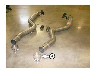
8. Place **Y-pipe assembly (1)** into position behind front pipe and slide it into clamp until it stops. Support it with stand and tighten clamp enough to allow for adjustment. Y-pipe outlet with two bends should be oriented to drivers' side of vehicle.
