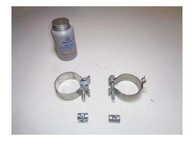
7. Transfer hangers from factory exhaust to Flowmaster muffler assemblies. Place clamps (4) (x2) onto inlets.
