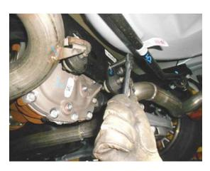
4. Loosen bolts (x2) at clamp connection in center of vehicle. Lift clip then with help, slide exhaust system back and off front pipe onto ground. The clamp should remain on factory front pipe for later use.
