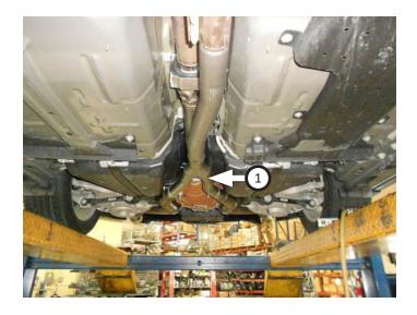
9. Connect **right muffler assembly (3)** to Y-pipe. Support assembly then remount rear hanger mount to frame. Remount front hanger to cross member. Repeat step with **left muffler assembly (2)** on left side of vehicle.
