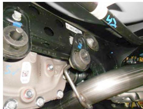
10. Adjust and level mufflers for a satisfactory fit. Maintain a minimum of ½" clearance around all components of exhaust system, keeping in mind suspension, travel and vibration. After making any required adjustments, securely tighten all clamps.
