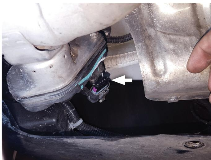
6. Remove bolts (x3) and detach actuator from mount. Retain bolts for later use.
