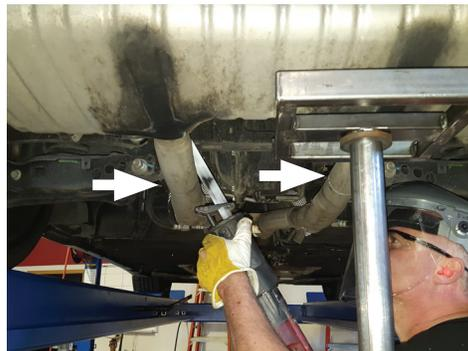
4. Remove screws (x4) attaching lower cover to frame to Mark factory driver and passenger tailpipes, 1" in front of bend as indicated.
