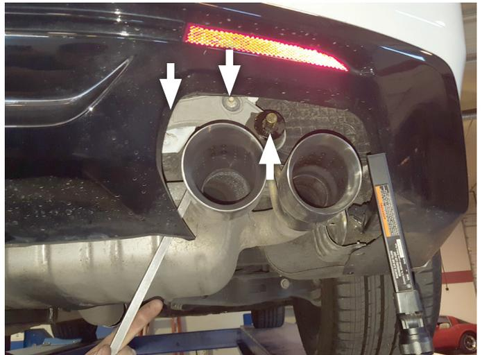
8. Dismount remaining wire hangers (x2) from isolators to remove factory muffler entirely from vehicle. Then remove muffler/pipe hangers from muffler and index them to their respective sides.
