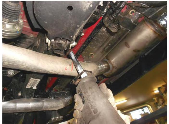
2) Begin by measuring back 1½" from the rear of the suspension cross-member shown in the photos above and make a mark on both pipes. Support the exhaust system both in front and behind the area to be cut, then once you've double checked that the measurements are correct, cut both pipes at the marks. **Note: Use caution when cutting!**
