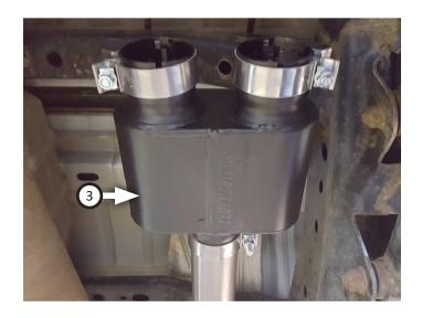
Route right (4) and left front tailpipes (5) over axle and connect them to muffler. Hang wire hangers into isolators and tighten clamps (x2) just enough to allow for later adjustment.
