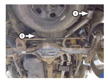
11. At rear of frame on driver side of vehicle (next to spare tire), is a pair of attached hanger mounts. Place **rubber hanger (11)** onto inner hanger.
