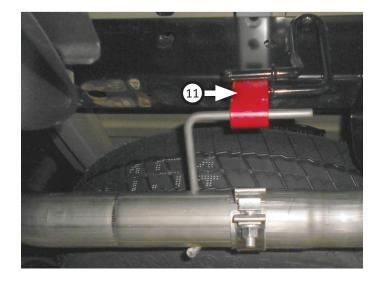
Place clamp (10) on left rear tailpipe (6) then connect it to left front tailpipe. Insert wire hanger into rubber hanger then tighten clamp just enough to allow for adjustment.
