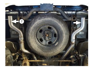
14. Place **stainless tips (9)** onto exit pipes and tighten inlets. Rotate exit pipes and tips to desired distance from body or bumper, so angle cut on tips are properly positioned.
