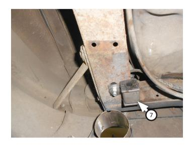
6. Fit **left muffler (5)** tip through left side bumper and insert wire hanger through bracket. Place **clamp (6)** onto muffler inlet. Repeat step with **right muffler (4)** and **clamp (6)** on opposite side.
