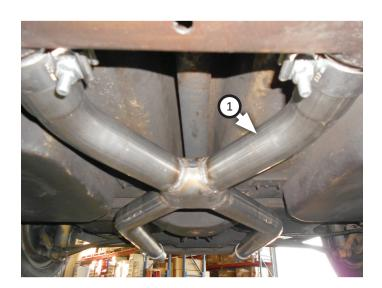
9. Adjust exhaust components for fit; maintaining ½" clearance and compensating for suspension, travel and vibration. Then fabricate downpipes down to connect x-pipe to factory exhaust.
