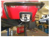
Place one of the supplied **HA602** rubber mounts onto the wire hanger of left muffler assembly **842456-352**. Place a provided clamp onto the muffler inlet, then place the assembly onto the back of the mid pipe and slide the two fully together. Support the muffler with a stand. Using a supplied 3/8" bolt, nut, washer and lock washer, bolt the **HA602** hanger to the hole in the frame above the muffler outlet.
