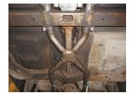
1) Starting just behind cross-member, place provided 2.25" clamp onto expanded ends of X-pipe assembly **86171S**, then slide it onto rear of manifold pipes (verifying connections are secure). Place stand under assembly rear and tighten clamps just enough allow for later adjustment.
