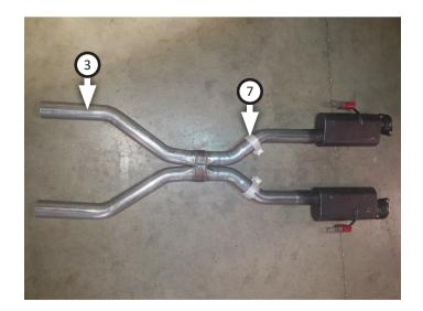
8. Place scavenger assembly into position to connect to factory exhaust. Set flanges together and secure mounts to vehicle frame with (x4) bolts (removed step 4).
