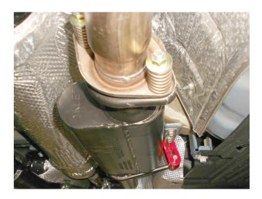
Place clamp (7) onto left muffler (4) then connect it to scavenger, inserting wire hanger into isolator. Tighten clamp just enough to allow for adjustment. Repeat this on passenger side with right muffler (5).
