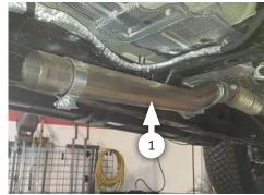
Place clamp (6) onto the mid pipe (2), situate the pipe over the axle, and connect it to the inlet pipe. Snug the clamp just enough to allow adjustment during system assembly.
