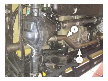
8. Fasten the **right hanger (4)** to the passenger-side frame studs with **2 lock nuts (14)**. Fasten the **left hanger (5)** to driver-side frame using **2 bolts (8)** and **flat washers (10)** inside the frame, and **2 lock washers (11)** and **nuts (9)** against the hanger. Install the **2 rubber hangers (7)** on the hanger rods.
