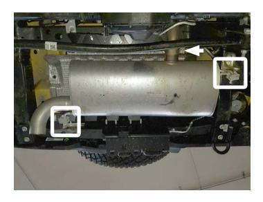
4. Support the front pipe, then remove the flange fasteners. Unbolt the isolator mount from frame, separate rear wire hanger from isolator, then remove front pipe from vehicle.
