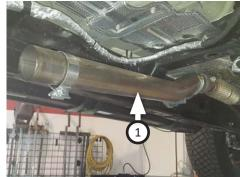
7. Place clamp (6) onto mid pipe (2) then route it ove axle and connect it to inlet pipe. Tighten clamp just enough to allow for adjustment.
