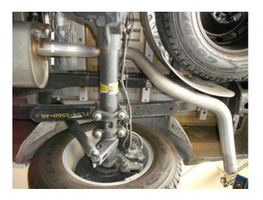
4. Support muffler and disassemble wire hangers from isolators. Remove and retain (x2 ea.) flange nuts and bolts, disconnect inlet pipe and remove exhaust system.
