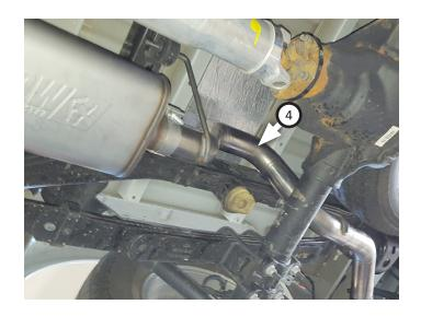
13. Place **tip (5)** onto muffler and tighten inlet. Rotate it to desired distance from body or bumper, so angle cut is properly positioned.
