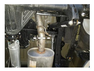
4. Support muffler and disassemble wire hangers from isolators. Remove and retain fasteners and gasket from flange, then remove muffler section from vehicle.
