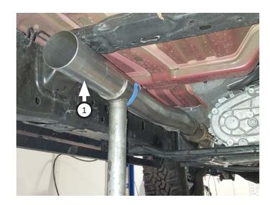
7. Place hanger mount (removed step 1) and clamp (3) onto muffler (2) then connect it to inlet pipe, inserting wires into hangers. Securing assembly by bolting mount to vehicle frame and tighten clamp.
