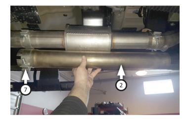
8. Place clamp (7) onto inlet pipe (1) then connect it to resonator delete pipe, straight tube or resonator pipe. Insert wire hanger in isolator and tighten clamp enough to allow for adjustment.
