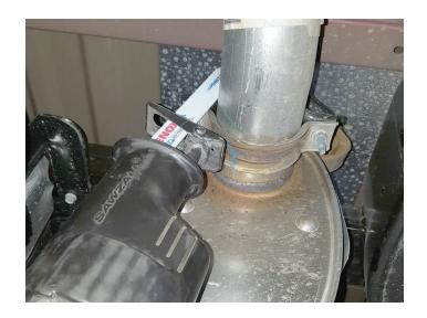
4. Remove clamp in front of muffler, then remove muffler section from vehicle.
