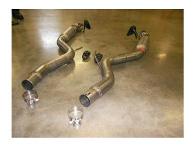
**NOTE:** The Y-Pipe outlet with two bends should be oriented towards driver side of your vehicle.
