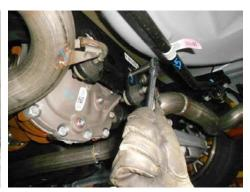
4. Loosen bolts (x2) at clamp connection in center of vehicle. Lift clip and with help, carefully slide system off of front pipe. Leave clamp on factory front pipe.
