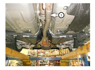
8. Connect **right muffler assembly (3)** 2" onto Y-pipe. Remount rear hanger mount to frame and front hanger to cross member then tighten them securely.
