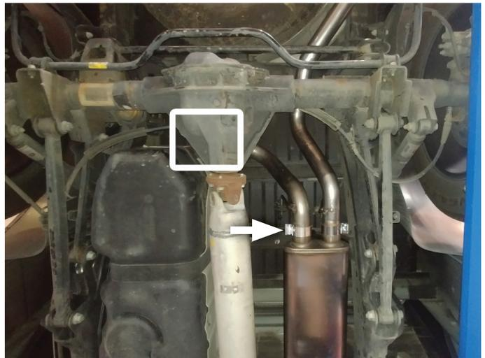
12. Place **clamp (8)** onto **left rear tailpipe (5)**, connect it to left front tailpipe and insert wire hanger in isolator. Tighten clamp just enough to allow for adjustment.
