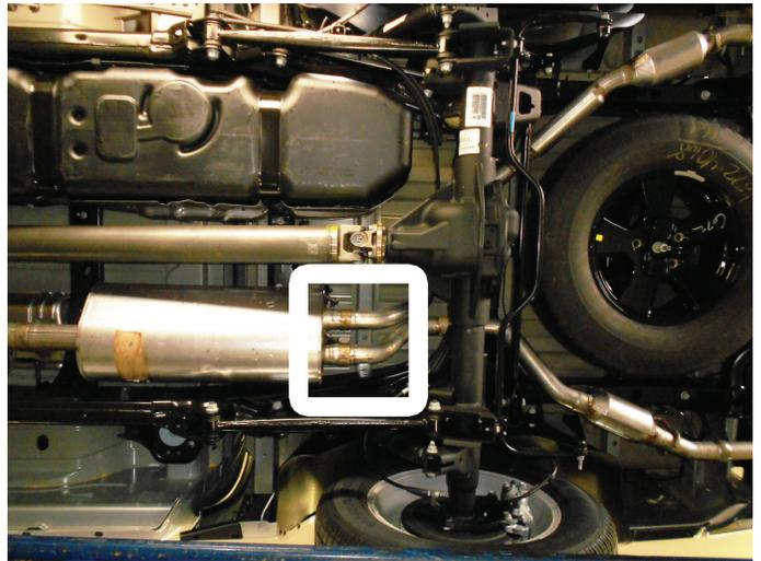
4. Dismount tailpipes from factory isolators (x3) and remove them from vehicle.
