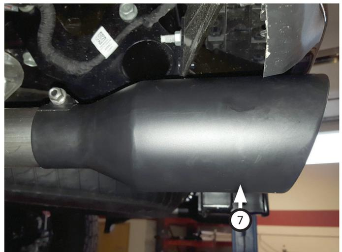
16. Adjust exhaust components for fit; maintaining ½" clearance and compensating for suspension, travel and vibration, then tighten all clamps.
