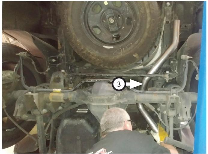
11. Remove isolator from factory mount (from step 4) and install it onto **left front tailpipe (4)**. Insert tailpipe wire hanger into factory mount then connect inlet to muffler. Tighten clamp just enough to allow for adjustment.
