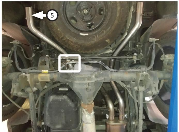
13. Place (x2 ea.) **clamps (8)** onto **exit pipes (6)** then connect them to tailpipes. Tighten clamps just enough to allow for adjustment.
