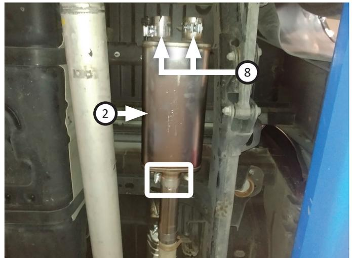
10. Route **right tailpipe (3)** over axle and insert wire hangers into factory isolators before connecting it to muffler. Clip in ground wire (removed step 5) then tighten clamp just enough to allow for adjustment.
