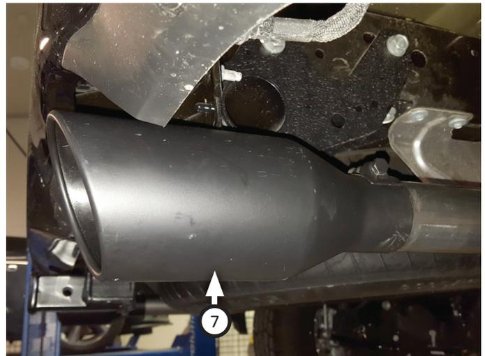
15. Place **tip (7)** onto driver side exit pipe. Secure it by fastening inlet bolt.
