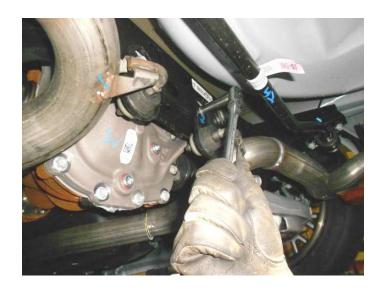
5. Loosen bolts (x2) at clamp connection in center of vehicle. Lift clip then with help, carefully slide exhaust system rearward out of hanger mounts and set it on floor. Leave clamp attached to factory front pipe.
