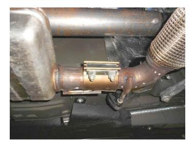
Transfer hangers from factory mufflers to FFX muffers and remove protective wrap. Remove nuts from stock and Flowmaster clamps, apply anti-seize compound to bolts and re-install nuts.
