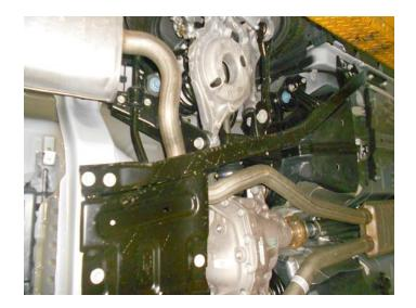
4. Unbolt hangers behind rear differential from cross member and at rear of vehicle from frame. Leave hangers attached to factory system for now.
