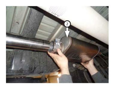
10. Transfer isolators from vehicle mounts to tailpipe assembly (3). Then route tailpipe assembly over rear axle and into muffler. Connect isolators to wire mounts and tighten clamps just enough to allow for adjustment.
