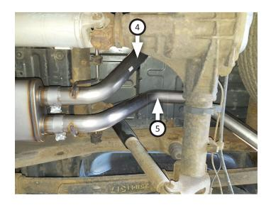
12. Place **clamp (14)** onto **left rear tailpipe (6)** then connect it to front tailpipe. Insert wire hanger into rubber hanger then tighten clamp just enough to allow for adjustment.
