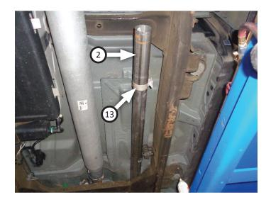
Place clamp (13) onto muffler (3) inlet then connect muffler to inlet/extension pipe. Place clamps (x2) (14) onto muffler outlets. Tighten front clamp just enough to allow for adjustment.
