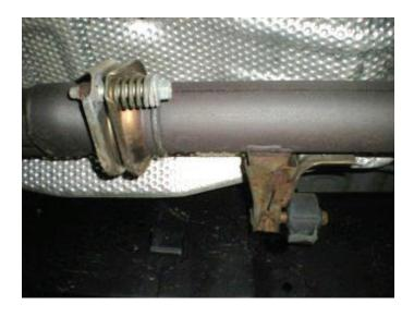
5. Separate (x4) hangers on muffler and front pipe assembly from rubber mounts on vehicle; then remove assembly from vehicle.
