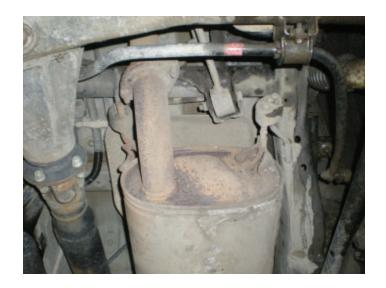
4. Remove (x2) factory spring loaded bolts at inlet pipe flange connection and set aside. Retain bolts and springs for later use.
