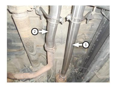
8. Place **left (6)** and **right (5) inlet pipe clamp hangers** onto inlet pipes then insert them into isolators. Tighten clamps enough to allow for later adjustment.
