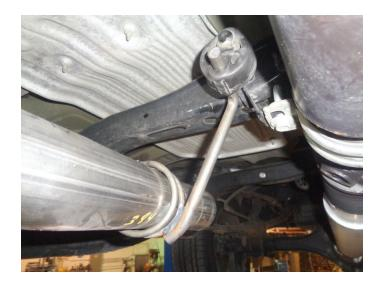
9. Place (x2) clamps (8) onto muffler (3) inlet then connect it to inlet pipes. Tighten clamps just enough to allow for adjustment.
