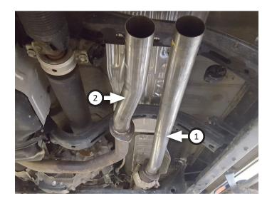
8. Slide **right (9)** and **left (11) inlet clamp hangers** onto corresponding inlet pipes and insert wire hangers into isolators on vehicle. Once in place, tighten clamps fully.
