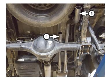
12. Place clamp (14) onto left rear tailpipe (6), connect it to left front tailpipe and insert wire hanger into rubber hanger. Tighten clamp enough to allow for adjustment.
