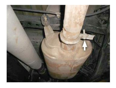
4. Unbolt bolts (x4) at both front flanged connections. Disassemble wire hangers from isolators then remove muffler assembly. Retain bolts for later use.
