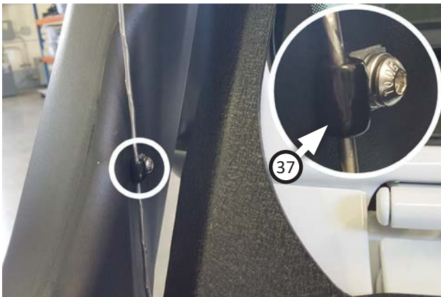
31. Place loom clamp (37) onto antennae, pinch it closed then secure it to snorkel using screw (38), lock washer (32) and flat washer (33).
