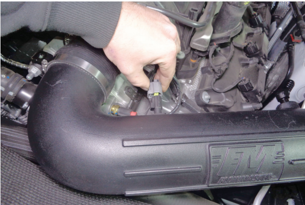
26. Plug connector into IAT sensor on intake tube.
