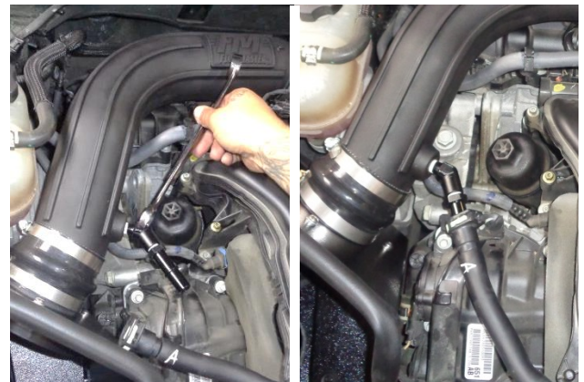
28. Align the elbow and quick connect fitting with the breather hose. Connect the breather hose to the fitting and verify the connection is secure.
