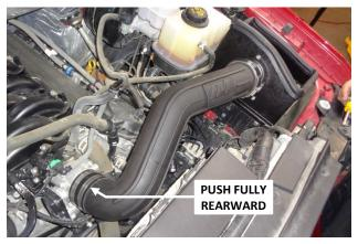
20. Push the straight coupling up against the throttle body and tighten the throttle body clamp. Then center the intake tube between the couplers (equal amounts of tube inserted in each coupler), and tighten the last two screw clamps.
