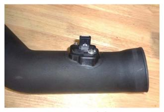
17. Place the MAF sensor gasket (12) over the sensor, ensuring correct orientation. Then install the sensor in the intake tube, using M4 screws (13).
