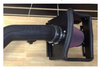
18. Assemble the intake tube and heat shield. Snug the tube clamp (do not tighten at this time).
