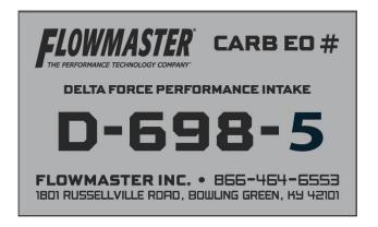
24. Affix the CARB Exemption Order label to a clean, readily-visible location under the hood (e.g., near the hood latch), so an inspector can easily see it at emissions testing.
