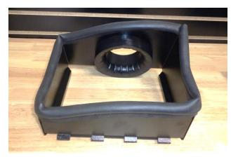
11. Attach the gasket (1) to the heat shield. Firmly press the gasket onto the heat shield, gradually working your way around. When you return to the starting point, use metal-cutting shears to trim the gasket to length.
