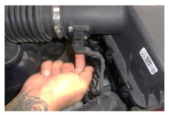
4. Disconnect the mass airflow (MAF) sensor plug by pulling the locking tab (on the bottom of the plug) away from the sensor until it stops, then pulling the plug straight off the sensor.
