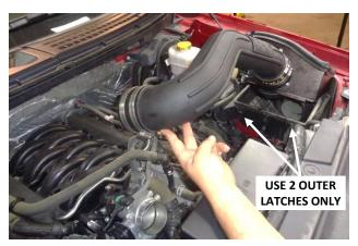
19. Insert the four tabs on the heat shield into the slots on the airbox. Lower the intake tube and install the straight coupling on the throttle body. Secure the heat shield to the airbox with the two outer latches. NOTE: The center latch is not used.
