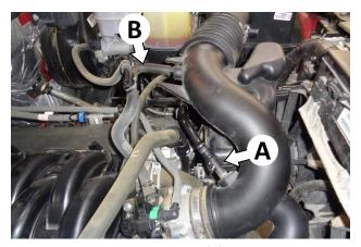
5. On the PCV hose connector (A), release the latch and disconnect the hose from the intake duct. Disconnect the EVAP hose (B) from both the intake duct and the check valve.
