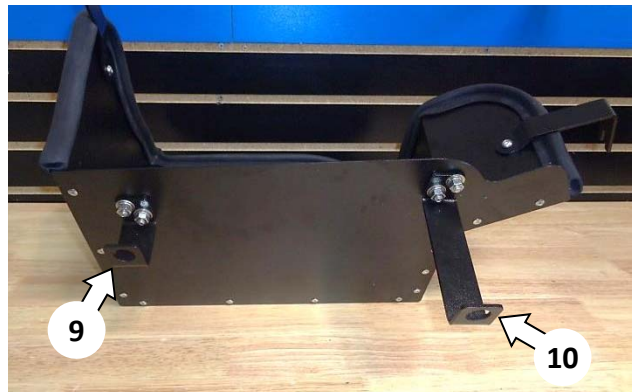
17. Attach brackets (9) and (10) to the heat shield as shown, using ¼-20 screws (8) and flat washers (4) (on the heat shield side), and lock washers (5) and nuts (6) (on the bracket side).
