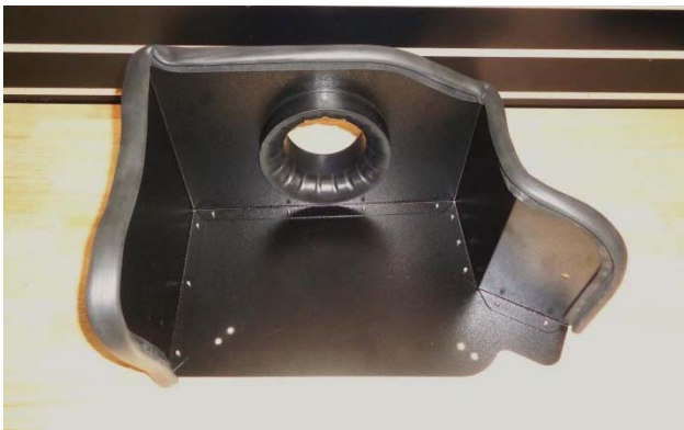
14. Attach the gasket (27) to the heat shield. Starting at one end, firmly press the gasket onto the edge, gradually working around the heat shield. When you reach the other end, trim the gasket to fit using metal-cutting shears.
