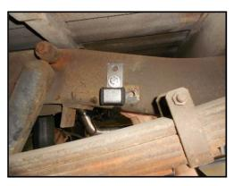
2) Locate the cross member at the front of the rear leaf spring, on the left side of this cross member, there will be a factory hole 9.00" in from the frame and  $\frac{3}{4}$ " up from the bottom, this hole location will need to be duplicated on the right side of the vehicle. Measure over 9.00" from the frame and  $\frac{3}{4}$ " up as shown in the photos below, use a center punch to make a mark and drill a  $\frac{5}{16}$ " hole on this mark.
