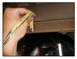
3) Remove the 5/16" hardware from the parts kit, place a 5/16" flat washer over the 5/16" bolt and place thru the hole in the **211HA** hanger as shown below. Place the hanger into position with the bolt thru the frame; place a second 5/16" flat washer over the bolt followed by a lock washer and nut. Make sure that the hangers are level and tighten securely. Place a **HA168** red exhaust isolator onto the end of each mount.
