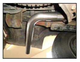
7) Included in the system are 2 different exit pipe styles, determine which of the exit pipes that you would like to use. Place a clamp over the expanded end of your chosen exit pipe and slide them onto the back of the over-axle pipes. Tighten the clamps enough to hold. **Note:** For short bed model trucks, 10.00" will need to be trimmed from the back of the rear exit pipes #86357.
