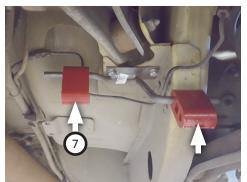
7. Thread (x2) **bolts (8)** into frame at both rear corners of vehicle. Use holes nearest center of vehicle.
