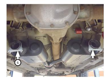
Route right (3) and left (2) tailpipes over axle and connect them to mufflers. Insert front wire hangers into isolators then tighten clamps just enough to allow for adjustment. **NOTE:** You may have to loosen other exhaust components to route tailpipes over axle and fit them in mufflers. If using a lift, jack up frame so you can fit tailpipes over axle.
