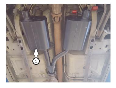
9. Place (x2) **clamps (6)** onto muffler outlets, leave them loose.
