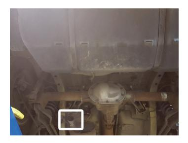
4. Remove fasteners and disconnect inlet pipe at catalytic converter. Disassemble wire hangers from isolators and remove muffler exhaust section from vehicle. Retain fasteners for later use.
