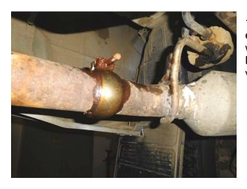
1) Locate the clamped connection just behind each of the factory exhaust tips, spray the clamp bolt with a penetrating lubricant and allow to soak. Loosen the bolts and remove the factory tips from the vehicle.
