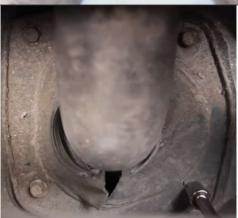
Remove the filler neck seal – Remove the four 10mm screws that hold the rubber seal to the trunk floor.
