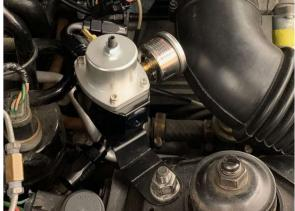
Mount the regulator in the orientation shown to the strut tower bolt shown.
