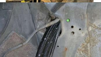
Route the hoses into the engine bay via the hole in the passenger wheel well shown.
