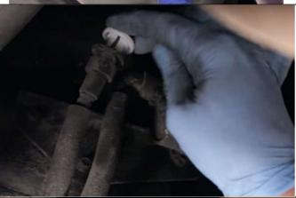
Remove the return line -- Using a quick disconnect tool remove the return soft line from the chassis hardline. Make sure to have a drain pan in place to catch any gas.
