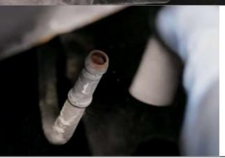
Remove the vapor line -- Remove the vent vapor line from the hardline. There should be no gas that comes out of here.
