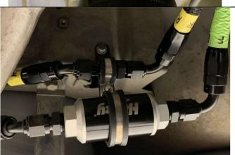
Mount the post filter and return bulkhead – Using the factory bolt and mounting location shown mount the post filter and return bulkhead.
