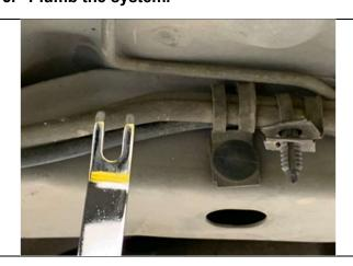
Remove the Factory Fuel Lines – The plumbing for this kit uses many of the factory fuel line mounting positions so the factory lines and filter must be removed to do this there are some fir tree mounts that must be removed as well as some rivets that need to be drilled out.
