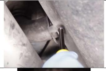
**Remove filler neck support** – Remove the single 5/16 retaining screw that holds on the filler neck support.
