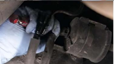
Remove the feed line -- Using a small flat blade screwdriver, remove the clip that holds the supply line to the fuel filter then remove the line. Again, be sure to have a drain pan in place to catch any gas.
