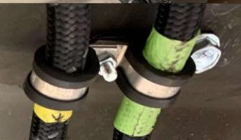
Using one of the three thinner flat drop links, two of the 3777G clamps, and one of the six screws and locknuts found in the 85R kit create a mount for the hoses to route through as shown.
