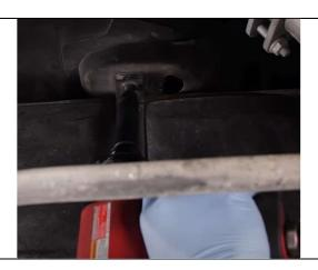
Remove the Filler Neck – In many cases at this point the filler neck can be removed at this point with the help of some lubrication. Sometimes you can just wiggle it right out, but other times the tank may need to be dropped slightly.
