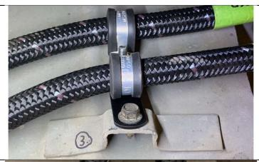
Using one of the three thinner flat drop links, two of the 3777G clamps, and one of the six screws and locknuts found in the 85R kit create a mount for the hoses to route through as shown. The factory mounting position and bolt will be used.
