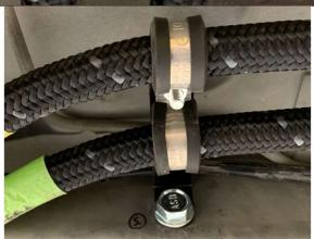
Route the hoses along the front frame rail then using one of the 90-degree brackets two of the 3777G clamps, and one of the six screws and locknuts found in the 85R kit create a mount for the hoses to route through as shown.
