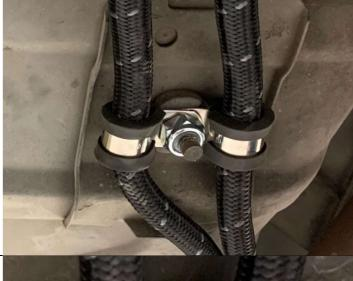
Using the two loop clamps in the 85R kit with the large diameter mounting holes and the large diameter locknut in the kit create a mount for the hoses to route through.
