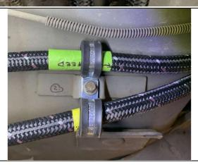
Using the factory mounting position and bolt shown and two of the 3777G clamps create a mount for the hoses to route through.
