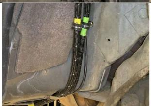
Using one of the 90-degree brackets, two of the 3777G clamps, and one of the six screws and locknuts found in the 85R kit create a mount for the hoses to route through as shown.
