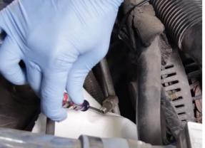
Relieve the system pressure -- Access the fuel Schrader valve on the feed line in the engine bay. This is located behind the alternator on the passenger side. Remove the cover, place a rag or towel under the valve, and depress the valve using a small screwdriver.
