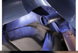
If the filler neck could not be removed earlier, then it can be now. Lower the tank slightly and move it over to the driver's side of the car. Then grab hold of the filler neck and wiggle it out of the tank.
