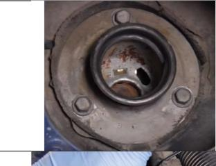
Unbolt the filler neck -- Open the fuel door, remove the fuel cap, and remove the three 10mm retaining screws that hold the filler neck to the filler box.
