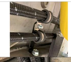
Continue routing the hoses down the front frame rail then using one of the 90-degree brackets two of the 3777G clamps, and one of the six screws and locknuts found in the 85R kit create a mount for the hoses to route through as shown.
