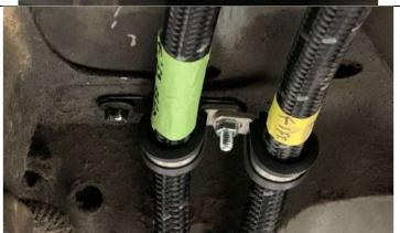
Create clamp mounts at factory locations – Using one of the three thinner flat drop links, two of the 3777G clamps, and one of the six screws and locknuts found in the 85R kit create a mount for the houses to route through as shown.
