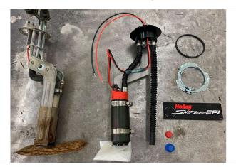
**Replace Fuel Pump Module** -- Remove the factory fuel pump module and follow the included instructions to install the new module into the tank. Be sure to lube the O-ring.
