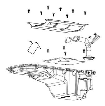
IMPORTANT: All gasket surfaces should be free of oil or other foreign material during assembly. Inspect the engine block oil gallery passages to make sure they are free from any debris or restrictions.
