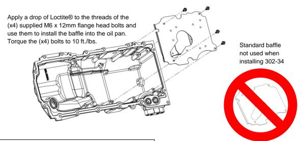
Reinstall the oil screen/pickup tube and gasket with supplied (x2) M6 x 16 flange head bolts. Apply a drop of blue Loctite® to the threads before installing. You may need to slightly adjust the bracket to provide precise alignment of the hole. Torque the bolts to 10 ft./lbs.
