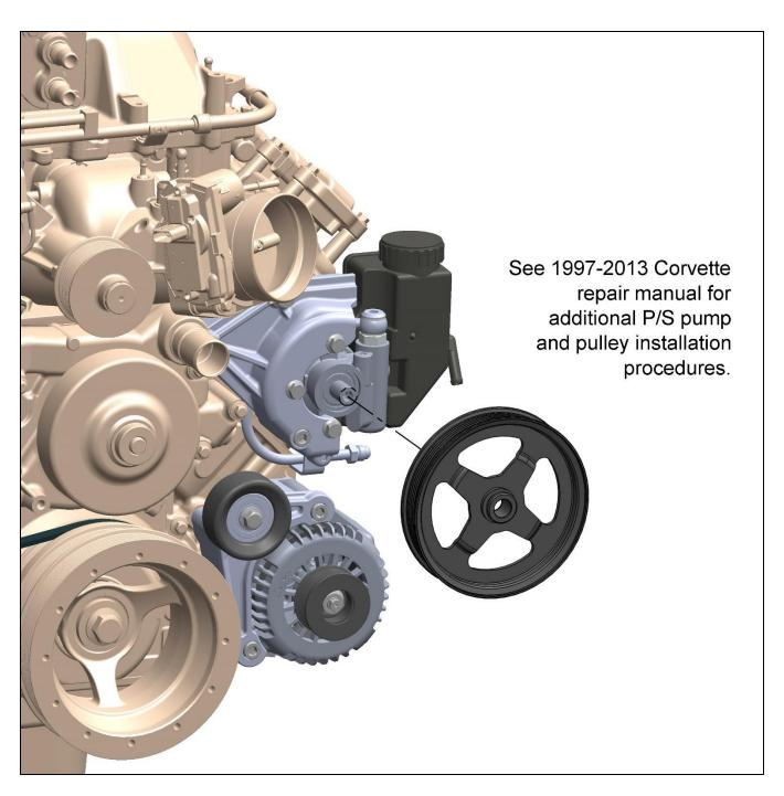
The P/S pulley must be installed using an installation tool that can be rented at most auto parts stores. Incorrect installation of this pulley may damage the P/S pump internals. When installed, the pulley bore face should be flush with the end of the pump shaft.
